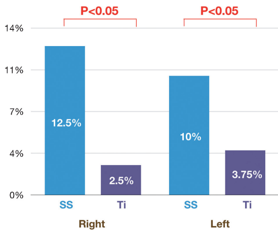
Fig. 9: For the right side, 12.5% ( \frac{1}{8} ) SS screws failed, but only 2.5% ( \frac{2}{80} ) Ti screws failed. For the left side, 10% ( \frac{8}{80} ) SS screws failed, and 3.75% ( \frac{3}{80} ) Ti screws failed. The red brackets document the differences were statistically significant ( P<0.05 ) on both sides.
