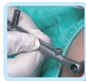
Fig. 4: The torque value to seat each incisal bone screw was measured with a clinical torque wrench.
